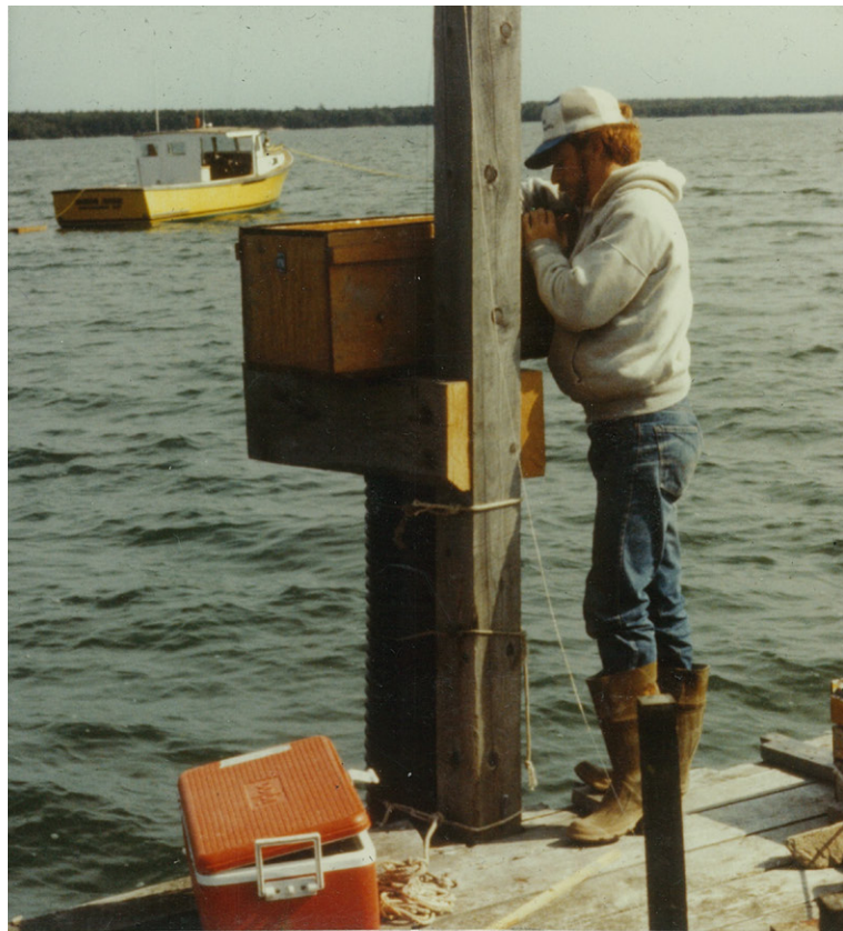
Figure 25. Tide station on lobster boat pier at the northwestern corner of the main bay.
