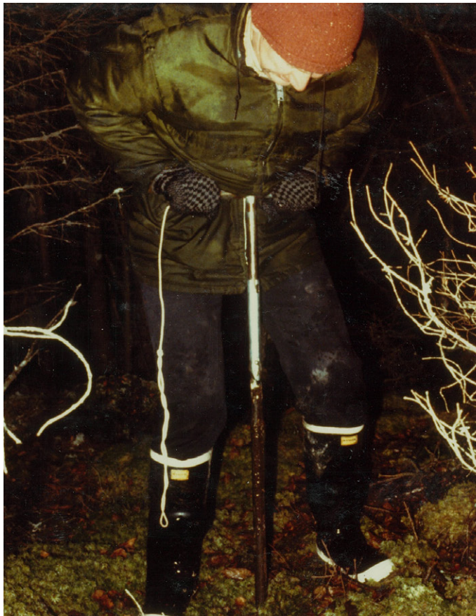
Figure 20. Auger coring for locations of Presumpscot clay near the forest/Great Marsh boundary.
