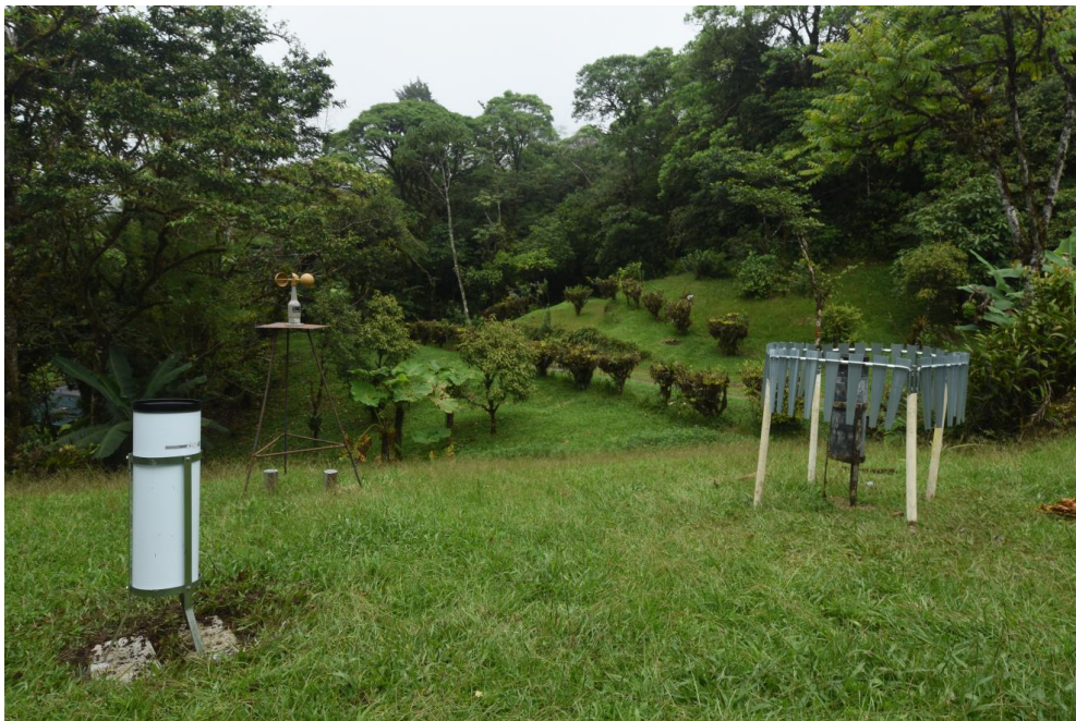
Figure 3. Original Rain gauge (right) with new wind skirt, and new rain gauge (left)
