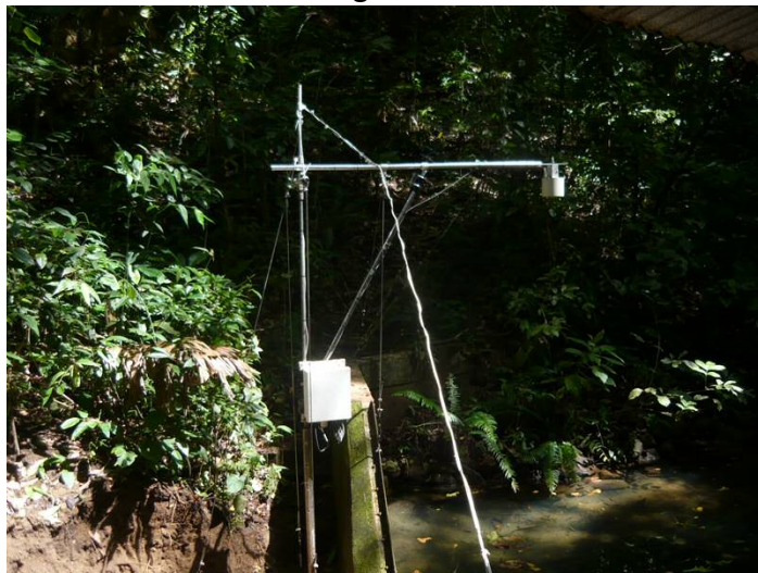
Sutron Radar device installed in 2014
