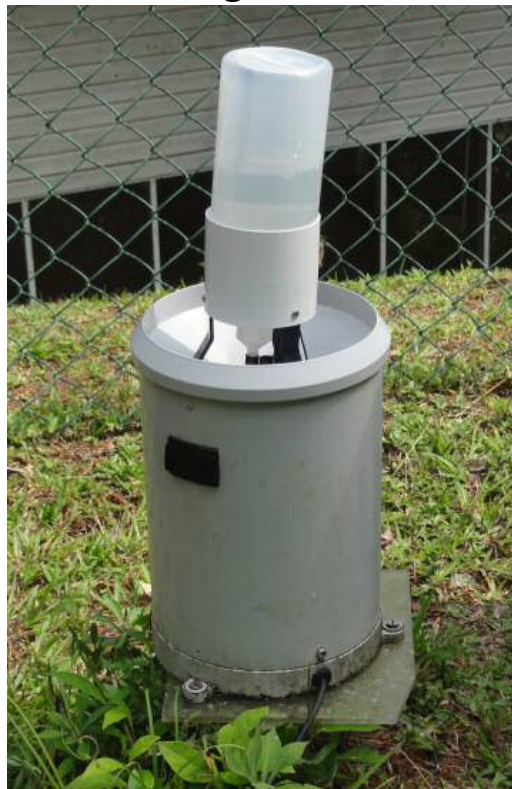
Tipping Bucket Calibration
