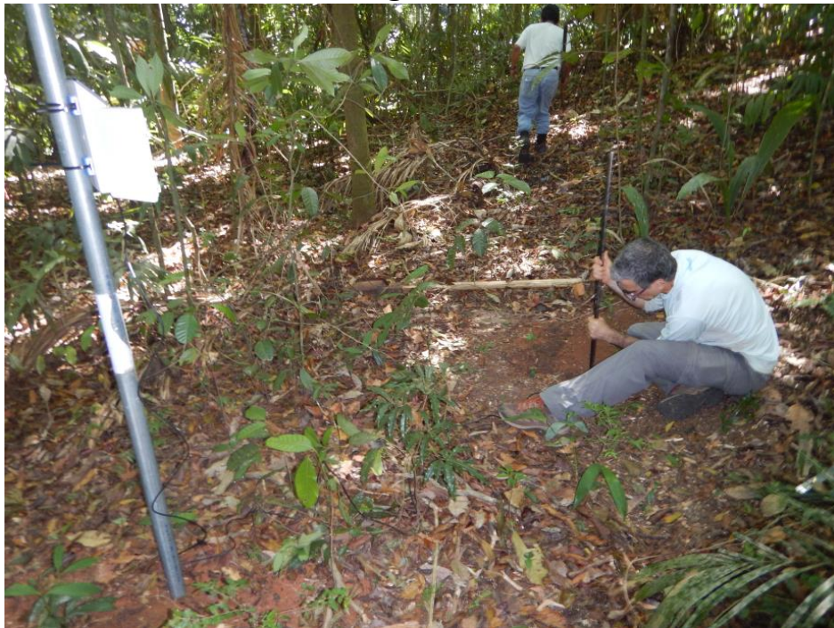
Installation of TEROS sensors
