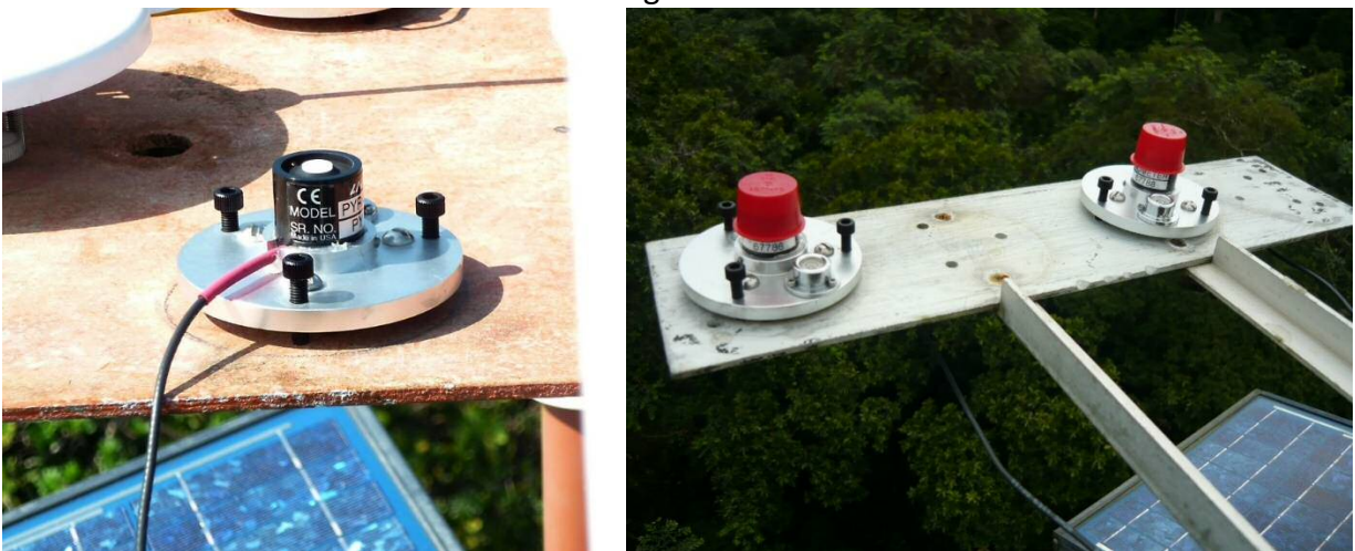
LiCor Model Li200x Pyranometers (with protective caps used during installation)
