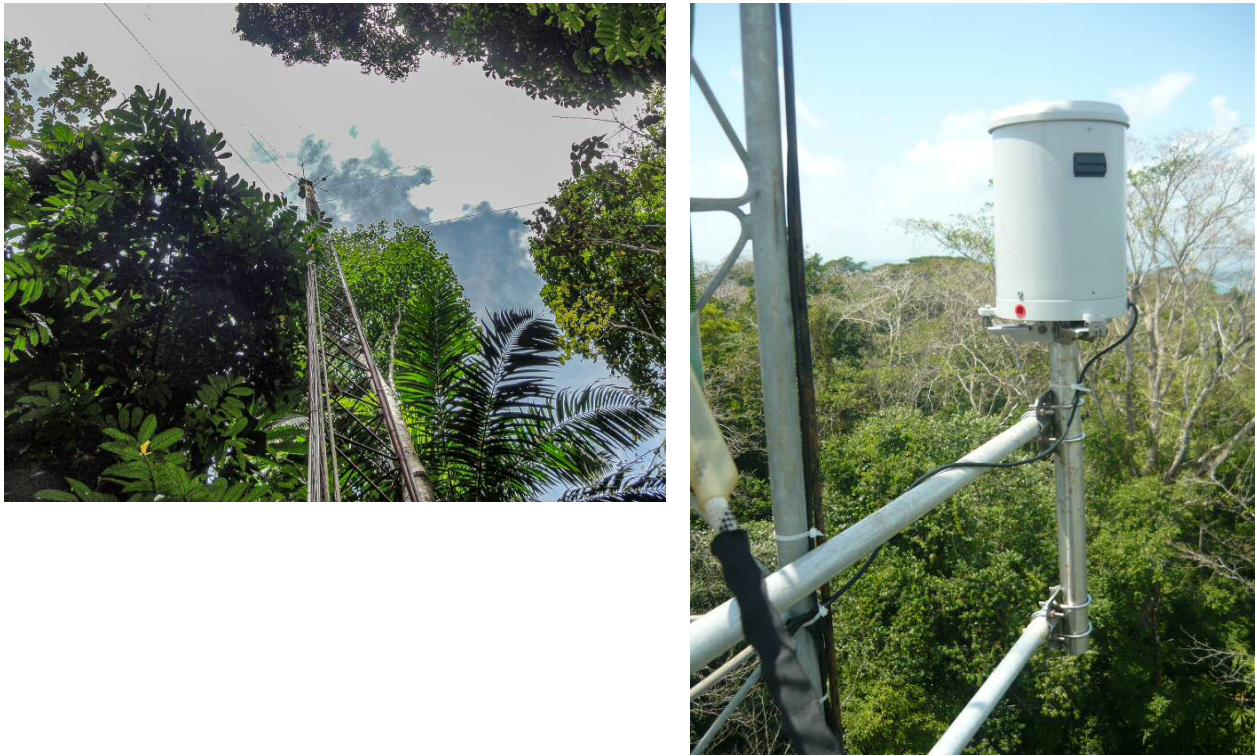
Campbell Sci. HygroVue10 Temperature & Humidity sensor inside 10-gill naturally aspirated radiation shield (left) and out (right)
