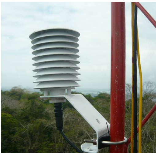
Campbell Sci. HygroVue10 Temperature & Humidity sensor inside 10-gill naturally aspirated radiation shield (left) and out (right)
