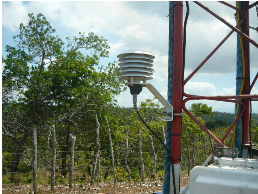
Campbell Sci. HygroVue10 sensor inside 6-gill naturally aspirated radiation shield
