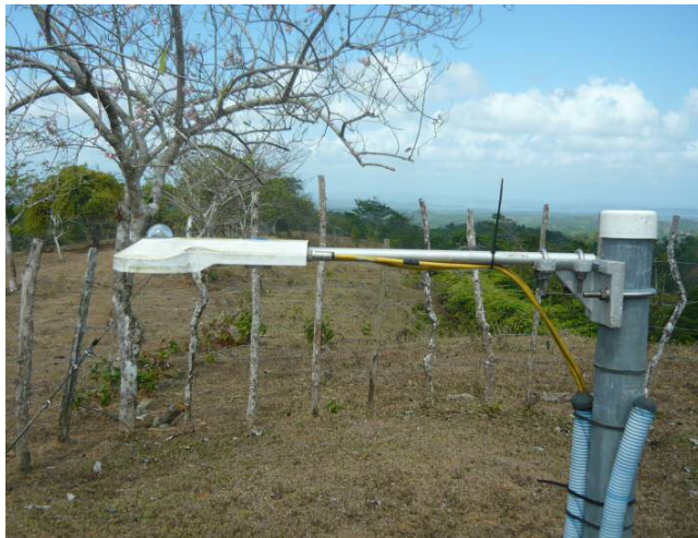
Installed CNR4 Net Radiometer (left) and close-up view (right)
