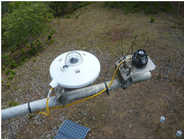
Kipp & Zonen PSQ1 Quantum Sensor at the end of pole (left) and close-up view (right)
