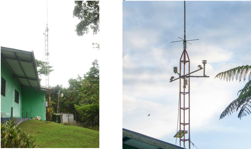
Radio tower (left) and close-up of solar radiation sensors located at either end of the cross-tube (right)
