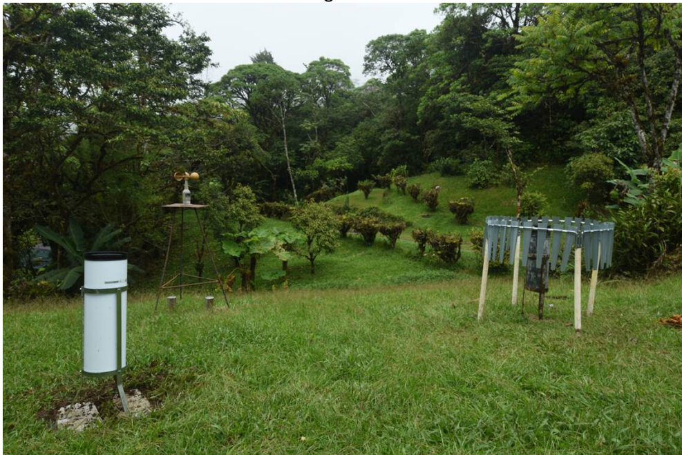
Original Rain gauge with new wind skirt (right), and new rain gauge (left)
