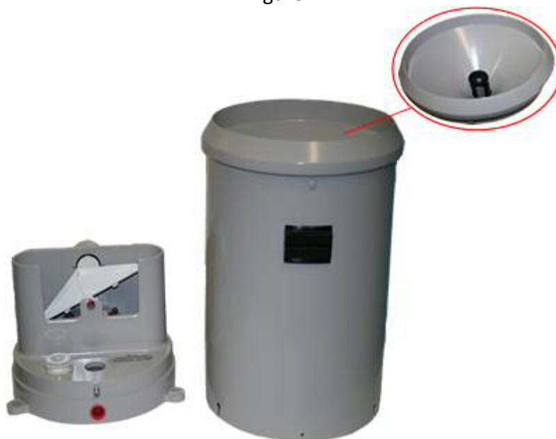
Hydrological Services Model TB4 tipping bucket
