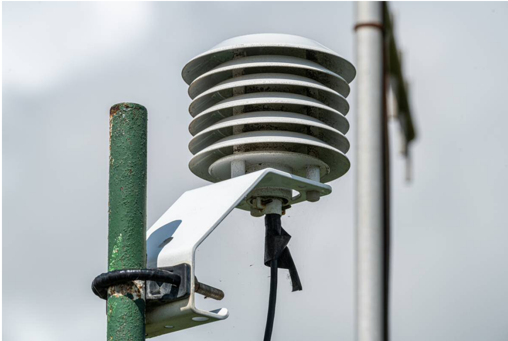
San Lorenzo Crane 6-gill radiation shield with sensor
