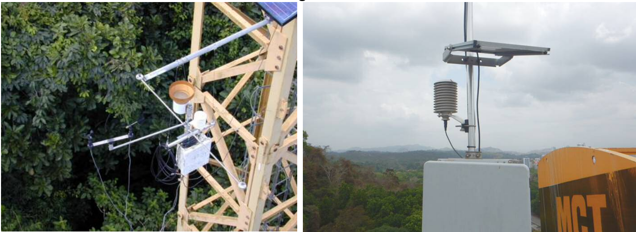
Original PNM tower showing original, 25m station (left) and new crane-top 10-gill radiation screen with sensor inserted from below (right)
