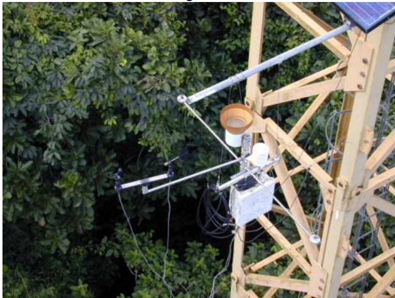
PNM tower showing met. station approximately at the middle of the tower (25m)
