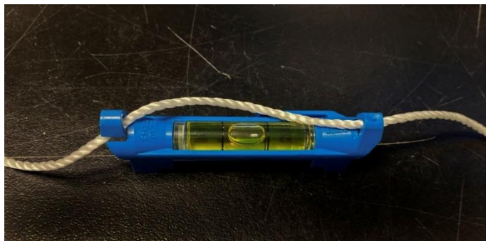
Figure 2: Line level used for reef height
