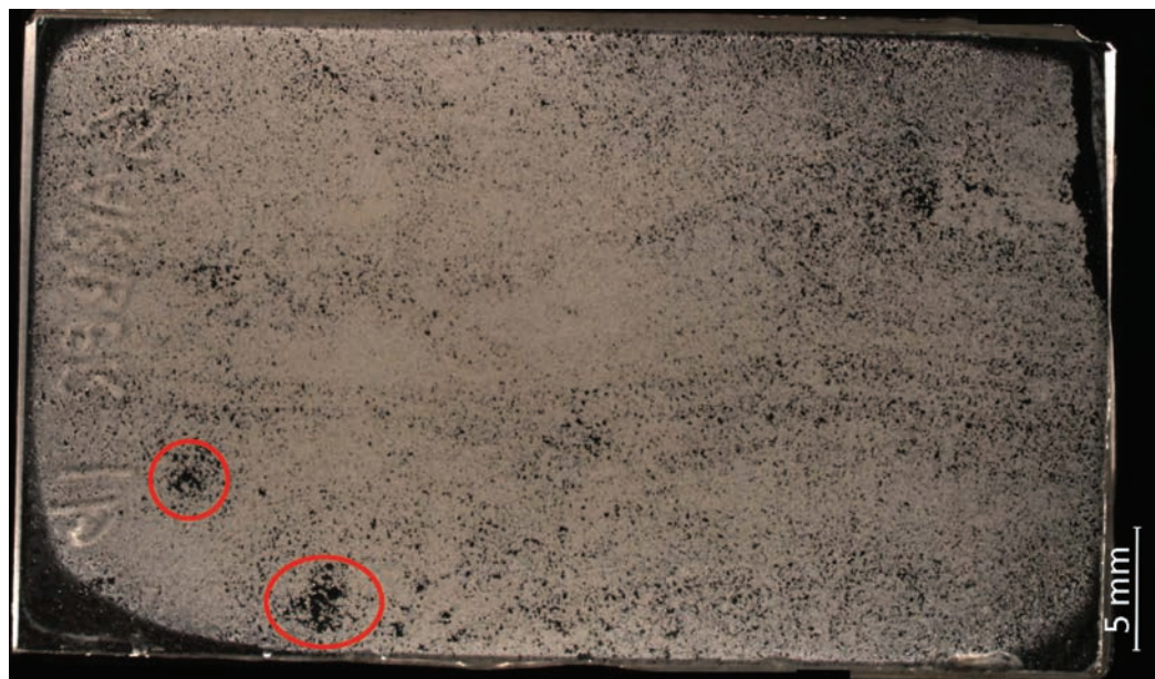
FIGURE 3. This dark-field image of an entire thin section of NMAI Kasota limestone (sample 1b) is a mosaic of five image tiles. Pores appear black in this image, and areas with the largest pores are circled in red. The largest pores measure about 1 mm (1,000 \mu\text{m} ) in linear dimension. Composite photo by Melvin J. Wachowiak, Smithsonian Institution.
