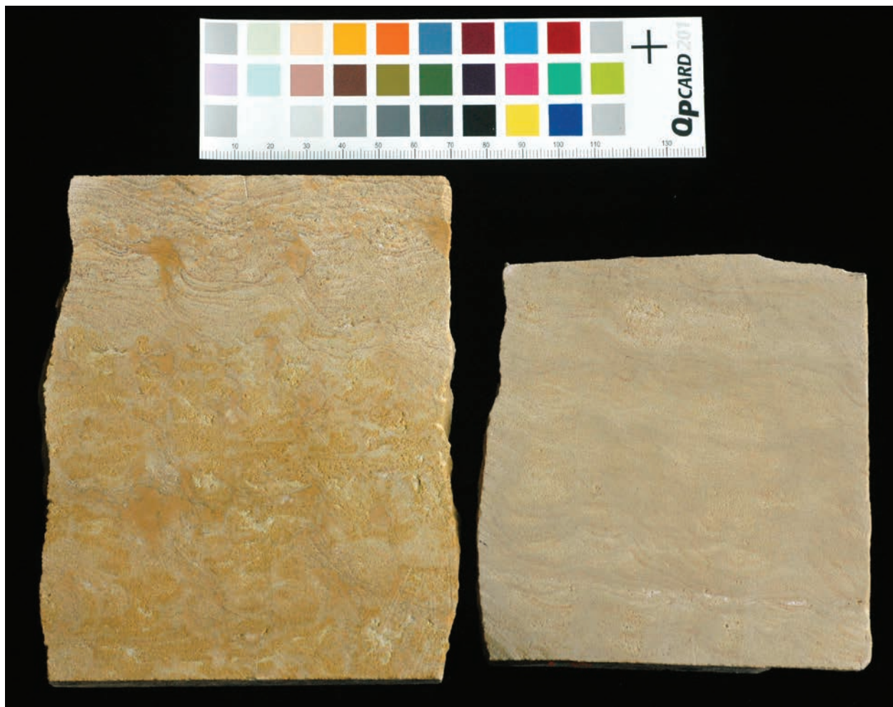
FIGURE 1. Cut surfaces of two wetted blocks of NMAI Kasota limestone showing differences in color and texture. Photo by Carol A. Grissom.
