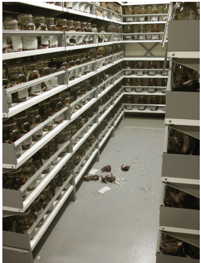
FIGURE 5. Jars on perimeter shelving had much less damage than those located in the central aisles of each alcohol storage bunker. (Photos by Suzanne C. Peurach, USGS Patuxent Wildlife Research Center.)
