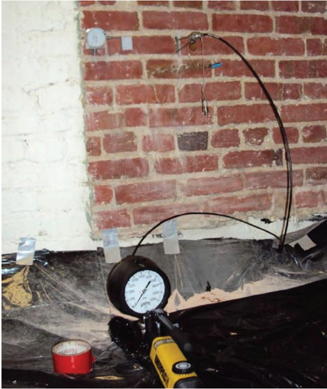
FIGURE 12. The shear stress wall test (left) is a fairly nondestructive test. The several slots made in the walls to place the flat plate jacks (right) are easily repointed after the test. This pressure test proved that the wall, which had shown no visible cracking after the earthquake, was not in need of reinforcement, which would have been an extensive, invasive, and expensive undertaking. (Photos: left, FMC & Associates; right, Sharon Park, Smithsonian Institution.)
