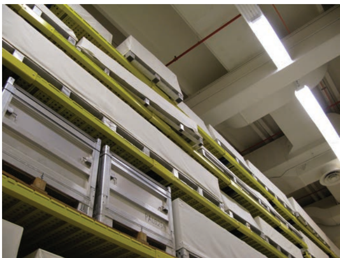
FIGURE 4. Walking of large palletized objects on cantilever shelves, in Pod 4. (Smithsonian Institution photo by David Rosenthal.)
