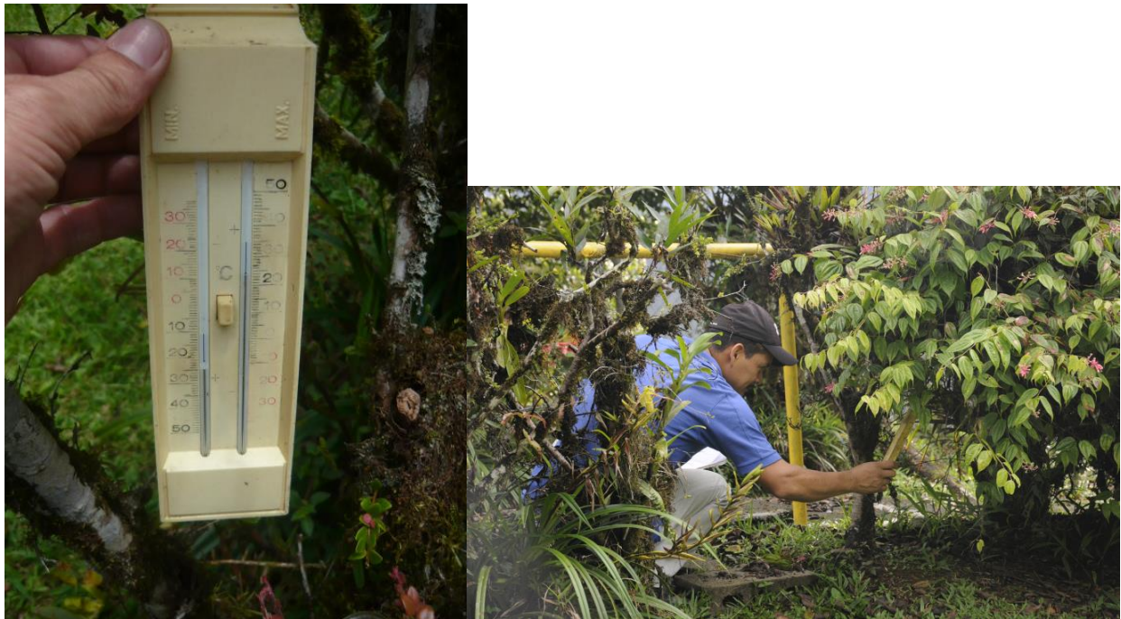
Figure 1. Max/Min Thermometer (left) and deployment location until March 31, 2016 (right)
