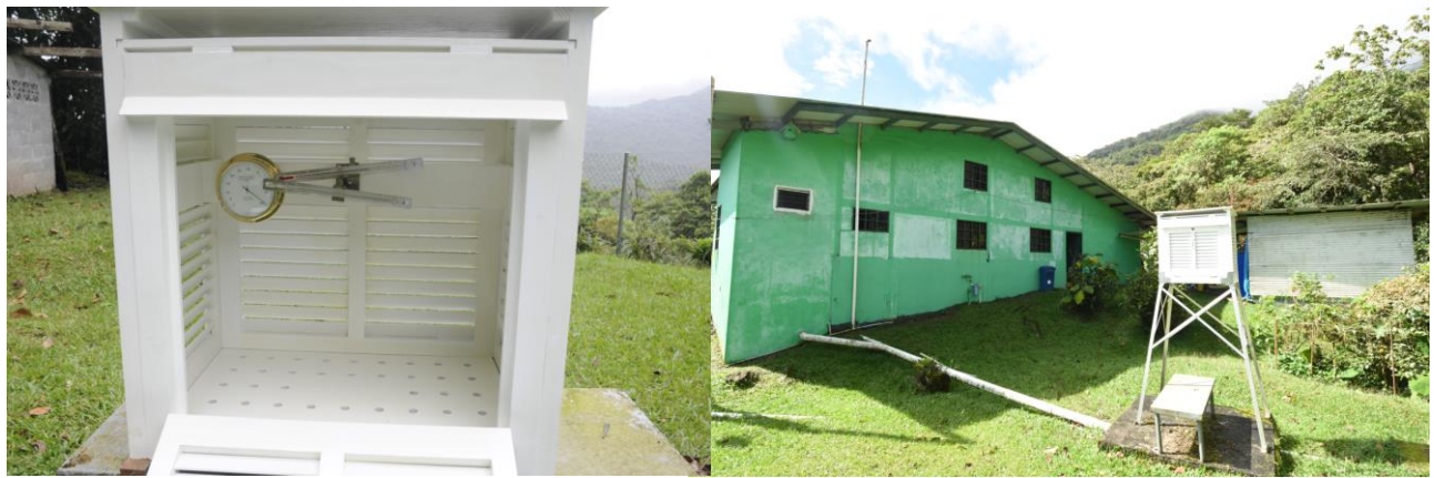
Figure 2. New Instrument shelter and Max/Min Thermometers
