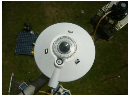
Currently, Celestino is the only station where both Photosynthetically Active Radiation (PAR) and solar flux (Pyranometer) is measured by STRI's Physical Monitoring Program.
